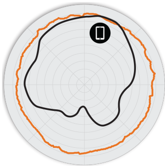
Figure 2. R850 2.4GHz Azimuth Antenna Patterns
